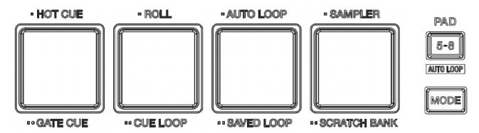
The first 4 pad modes can be accessed by holding the **MODE** button, and pressing the respective pad mode button once, and are as follows:
