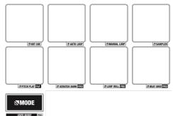
**HOT CUE mode**: Hold the **MODE** button and press **PAD 1** to select HOT CUE mode. In this mode pads 1-4 trigger Serato DJ Lite Cue points, and if no Cue point is present on that slot/pad, pressing that pad will set a Cue point. Holding down the **SHIFT** button while pressing a pad will delete the Cue point from the respective pad/slot.
