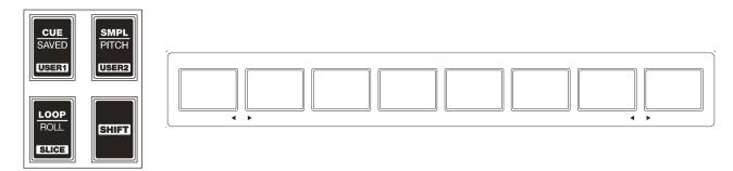
**CUE mode:** Pads 1-8 trigger Serato DJ Pro Cue points, and if no Cue point is present on that slot/pad, pressing that pad will set a Cue point. Holding SHIFT while pressing a pad will clear the Cue point from that pad/slot.
