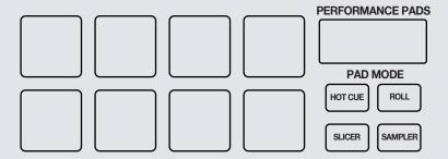
The Pioneer DJ DJM-S9 performance pads have eight different modes you can select. The first four modes are; Hot Cue, Roll, Slicer and Sampler. The second four modes, Cue Loop, Saved Loop, Slicer Loop and Sampler Roll are activated by holding SHIFT and pressing the respective performance pad mode buttons.
