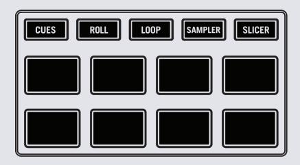
The performance pads have ten different modes you can select. The first five are activated by pressing the mode buttons once, the second five are activated by pressing the mode buttons a second time. For reference below the pads are numbered 1-8 from the top left pad moving to the right.
