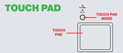
The KAOSS DJ **TOUCH PAD** has three different modes, **Controller Mode**, **Sampler Mode** and **KAOSS FX Mode**. Toggle through these modes by pressing the **TOUCH PAD MODE** button. Control the effect by rubbing or tapping your finger on the touch pad. Each axis (X,Y) will provide realtime control of a different effect parameter.
