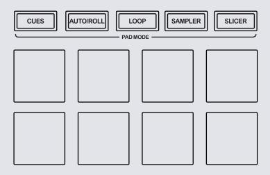
The performance pads have eight different modes you can select. The first four modes are; Hot Cue, Roll, Slicer and Sampler. For reference below the pads are numbered 1-8 from the top left pad moving to the right.
