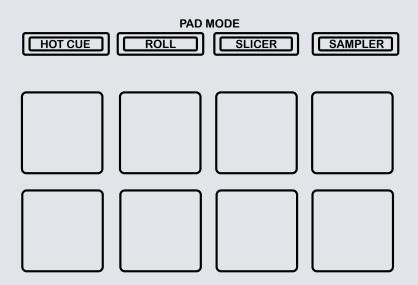
The performance pads have four different modes you can select. The four modes are; Hot Cue Mode, Loop Rolls, Slicer and Sampler.
