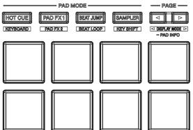
The first 4 modes can be triggered by pressing the performance pad mode button of the same name once, and consist of:
