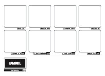
**HOT CUE mode**: Hold the **MODE** button and press **PAD 1** to select HOT CUE mode. In this mode pads 1-4 trigger Serato DJ Lite Cue points, and if no Cue point is present on that slot/pad, pressing that pad will set a Cue point. Holding down the **SHIFT** button while pressing a pad will delete the Cue point from the respective pad/slot.
