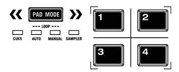
**HOT CUE mode**: Pads 1-4 trigger Serato DJ Lite Cue points, and if no Cue point is present on that slot/pad, pressing that pad will set a Cue point. Holding down the **PAD MODE** button while pressing a pad will delete the Cue point from the respective pad/slot.
