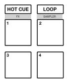
**HOT CUE mode**: Pads 1-4 trigger Serato DJ Lite Cue points, and if no Cue point is present on that slot/pad, pressing that pad will set a Cue point.
