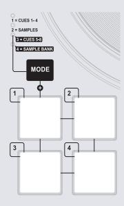
Choose the Performance Pad mode you want to use by holding the **MODE** button and pressing one of the 4 Performance Pads. Hold **MODE** and press Pad 1 for **CUES 1-4**, press Pad 2 for **SAMPLES**, press Pad 3 for **CUES 5-8** and press Pad 4 to choose **SAMPLE BANKS**.
