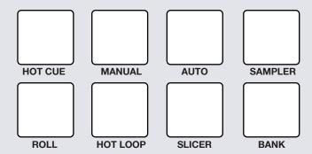
The performance pads have eight different modes you can select. **HOT CUE, MANUAL, AUTO, SAMPLER, ROLL, HOT LOOP, SLICER, and BANK.**
