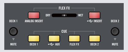
The FlexFx loop allows any combination of DECK 1, DECK 2, MIC or + C+ AUX to be assigned
